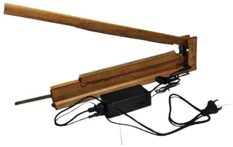
Gambar 1. Alat press plastik (sealer)
